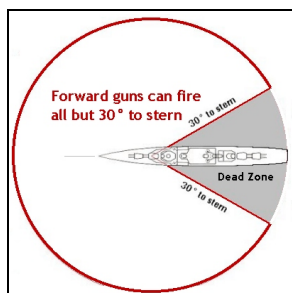
Turret No. 2 is blocked by superstructure (shaded region) shooting to the stern.
